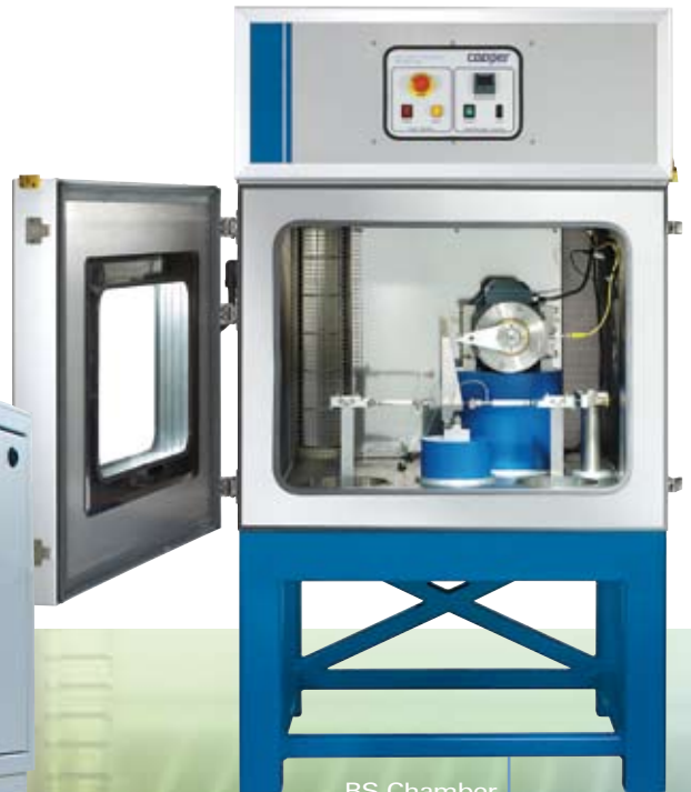
BS Chamber interfaced with a materials testing machine. Courtesy of Coopers Research Ltd.
