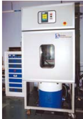
Electrodynamic vibrator interfaced in BS chamber floor.
