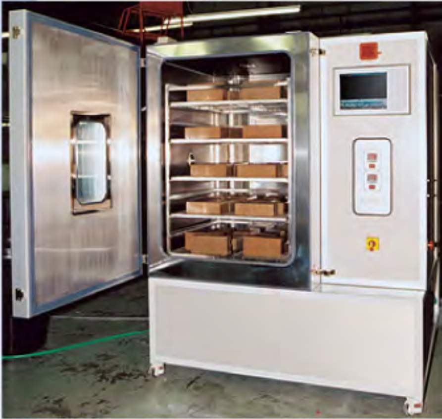
Customised 610 litre chamber designed to initially remove large quantities of water from the test samples over a set time and then maintain temperature and humidity levels within a close tolerance.
