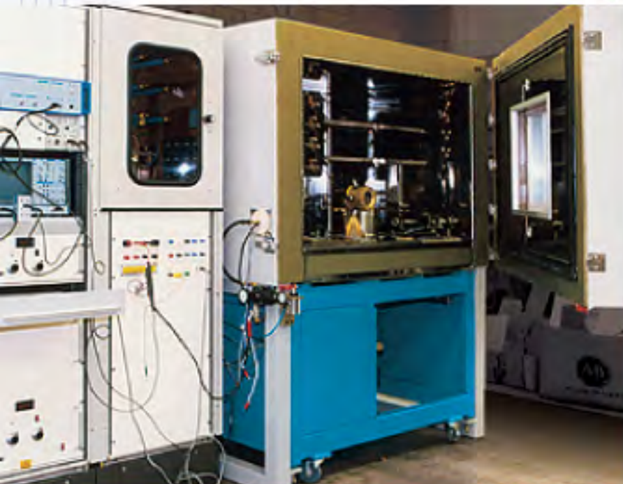
Temperature test chamber interfaced with automotive test rig. The chamber controls temperature to a close tolerance whilst counteracting heat input from the test item.
