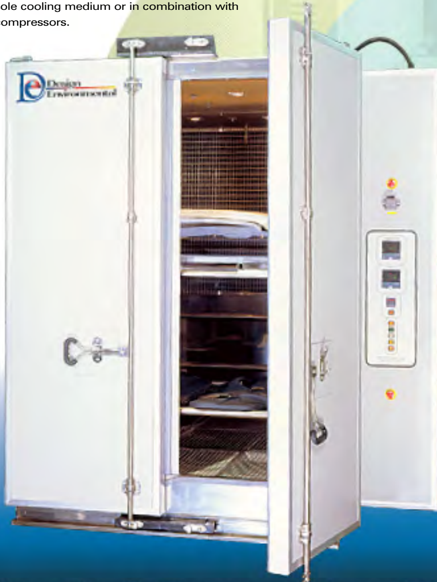
6,000 litre capacity chamber testing automotive roof liners and internal trim panels. Temperature range -40°C to +130°C with humidity 10-98%RH. A removable infrared lighting array can also be automatically linked to temperature.
